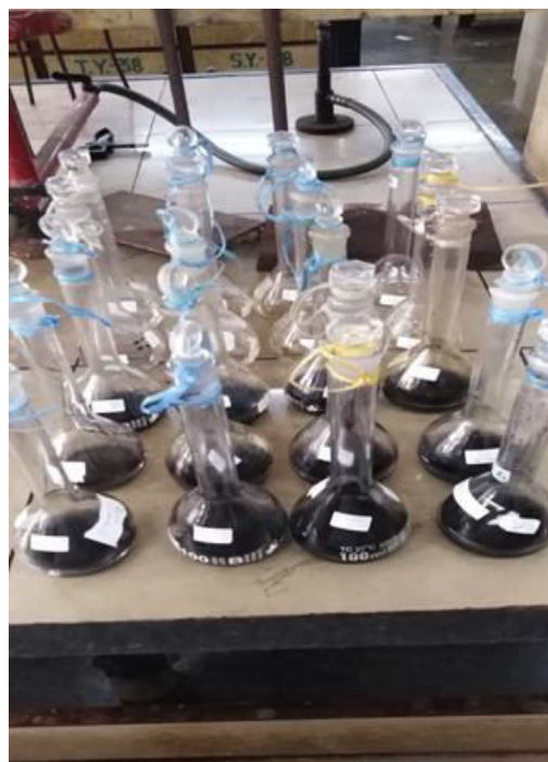
Picture (b): 100 cm 3 standard measuring flasks with adsorbent and fluoride solution before dilution
