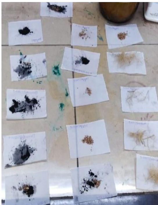
Picture (a): dried samples of Charcoal powder, apple peel powder, coconut husk powder
